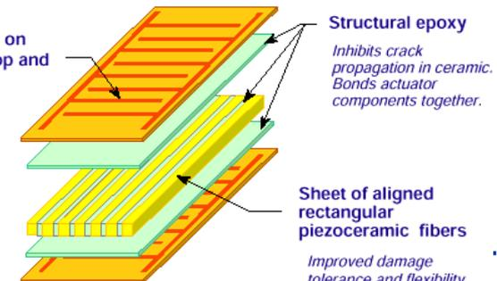
Improved damage tolerance and flexibility relative to monolithic ceramic.
