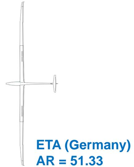
**Large aspect ratio for high aerodynamic efficiency**
