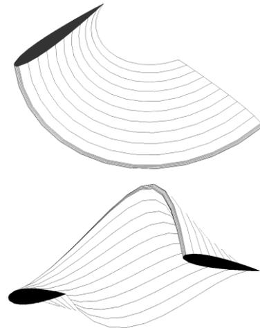
**Sample element deformations with constant strain**
