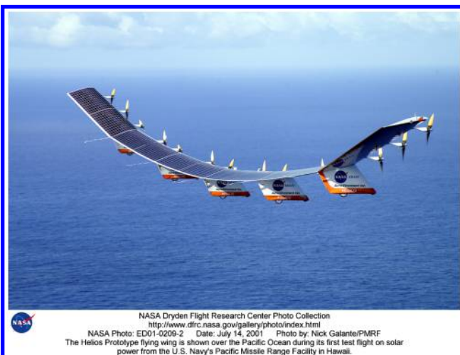
Fig. 1 Helios Prototype as a sample of highly flexible flying wing (photo courtesy of NASA Dryden Flight Research Center).
