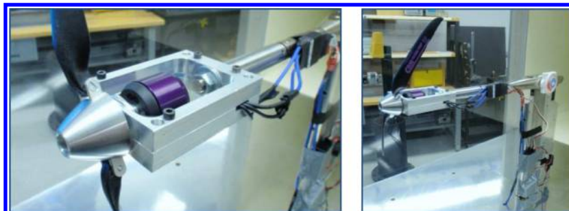
Fig. 17 2-ft-by-2ft wind tunnel test setup for calibration of the propulsion assembly.
