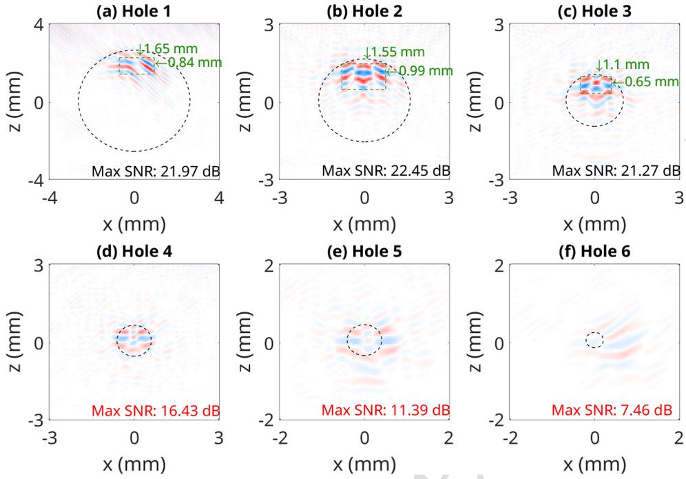
Figure 17: Zoomed in experimental steel images for each hole within  $K_{V_s}$ .
