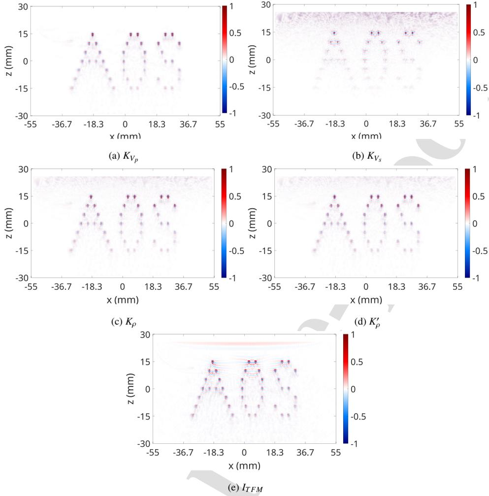
Figure 27: ARTM results for aluminum data with sensitivity kernels: (a)  $K_{V_p}$ , (b)  $K_{V_s}$ , (c)  $K_{\rho}$ , and (d)  $K'_{\rho}$ . (e) TFM Image.
