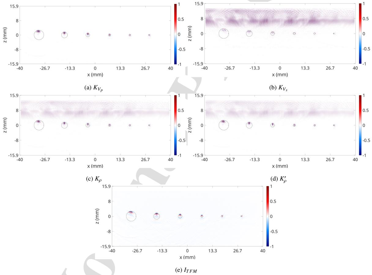
Figure 15: ARTM results for experimental steel data with sensitivity kernels: (a)  $K_{V_p}$ , (b)  $K_{V_s}$ , (c)  $K_{\rho}$ , and (d)  $K'_{\rho}$ . (e) TFM Image.
