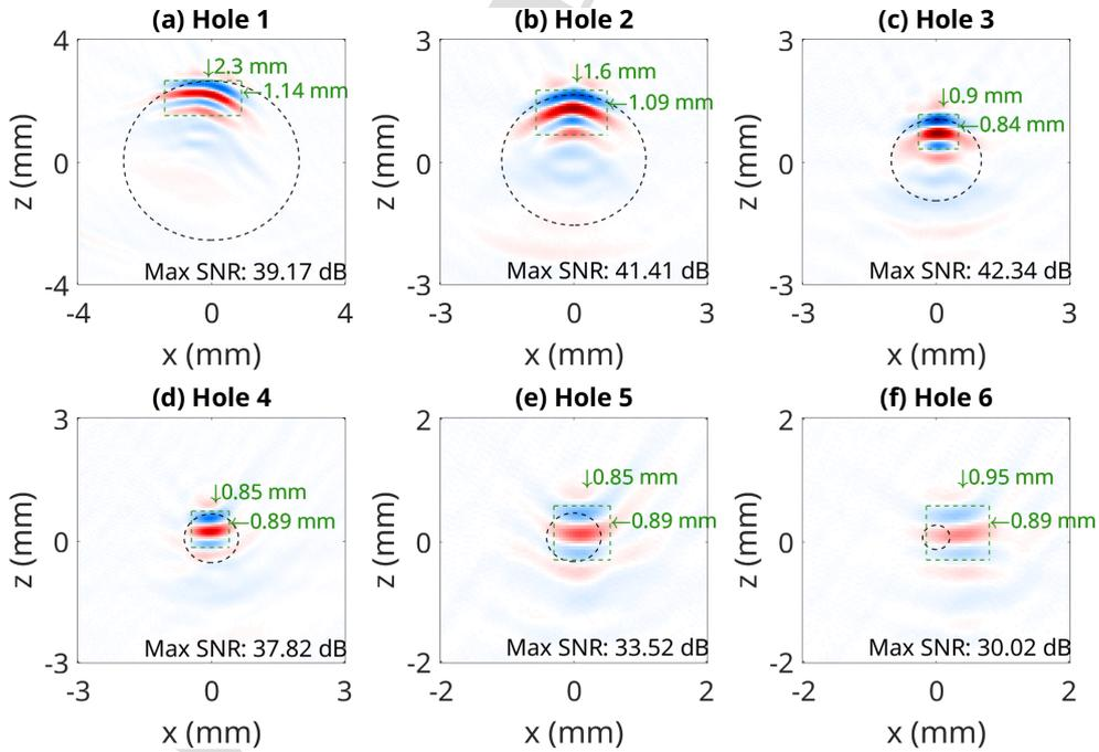
Figure 20: Zoomed in experimental steel images for each hole within  $I_{TFM}$ .
