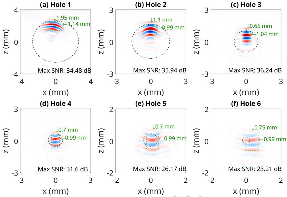
Figure 19: Zoomed in experimental steel images for each hole within  $K'_p$ .
