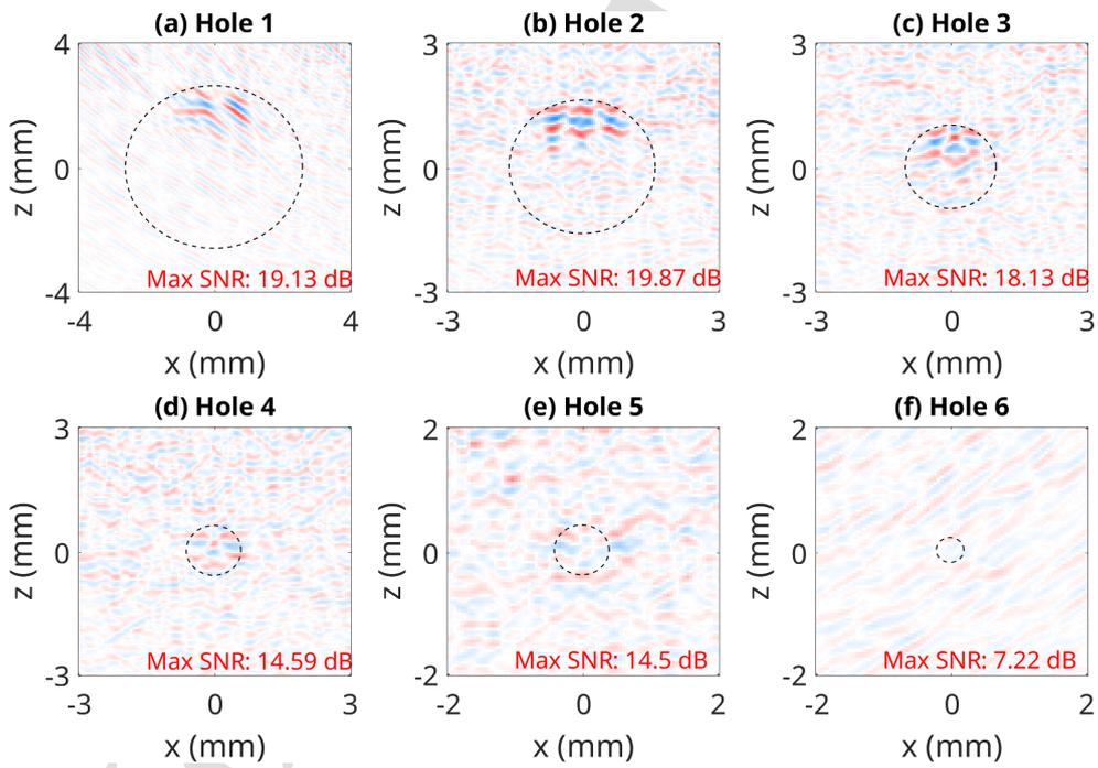
Figure 23: Zoomed in Experimental Steel Images for each hole within:  $K_{V_s}$
