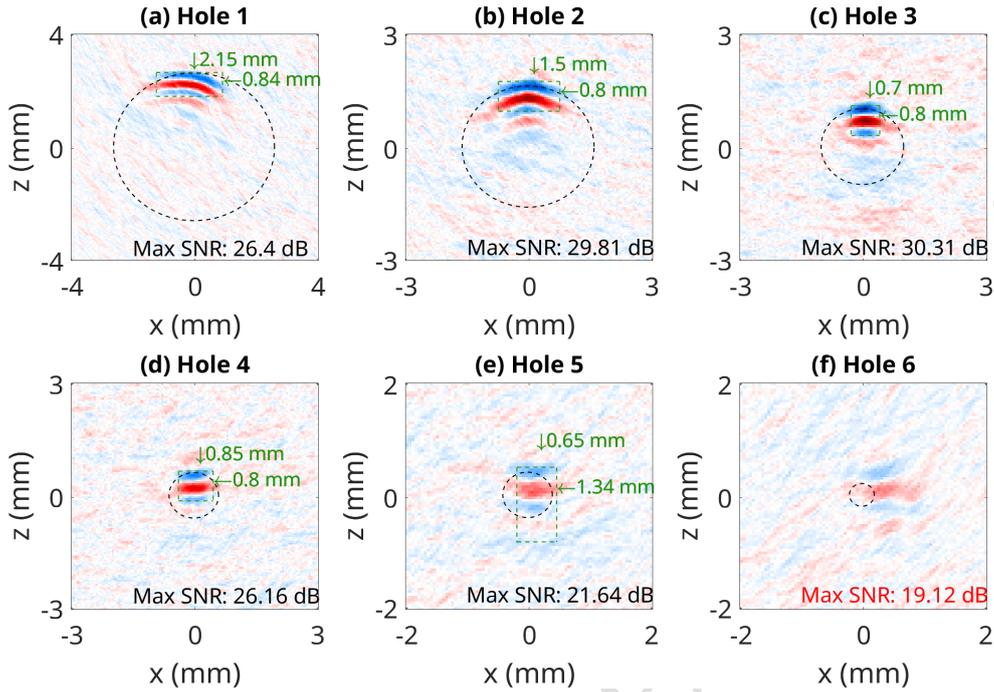
Figure 26: Zoomed in Experimental Steel Images for each hole within:  $I_{TFM}$
