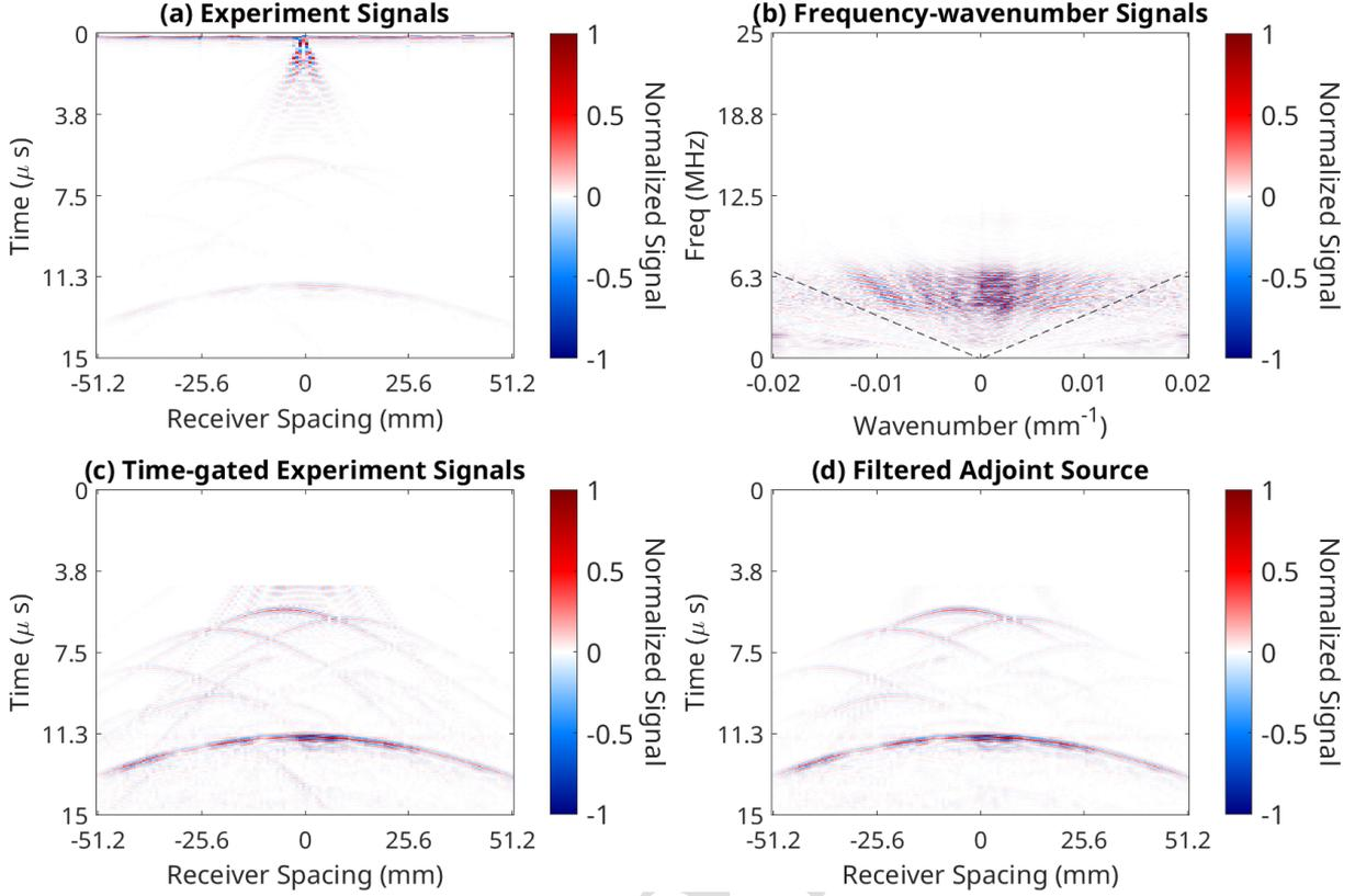
Figure 6: Example filtering of 5 MHz ultrasound data for source 64. (a) Unfiltered time-domain signals and (b) frequency-wavenumber signals and filtering zone. (c) The time-domain signals with time gating. (d) The fully filtered adjoint source.
