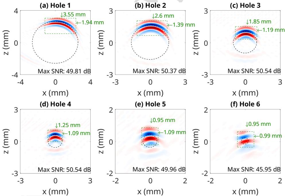
Figure 10: Zoomed in numerical steel images for each hole within  $K_{V_p}$ .
