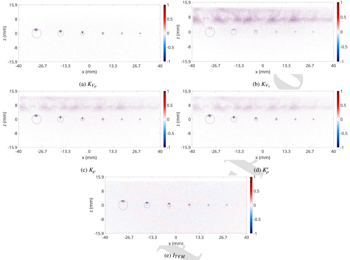
Figure 21: ARTM results for “noisy” experimental steel data with sensitivity kernels: (a)  $K_{V_p}$ , (b)  $K_{V_s}$ , (c)  $K_\rho$ , and (d)  $K'_\rho$ . (e) TFM Image.
