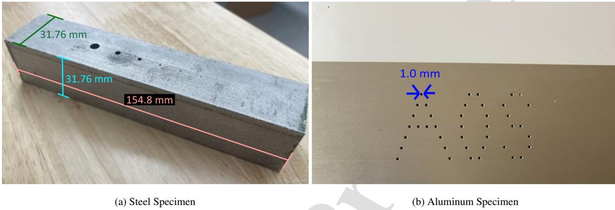
Figure 1: (a) Steel block with decreasing hole size. (b) Aluminum Block with "AOS" hole pattern.
