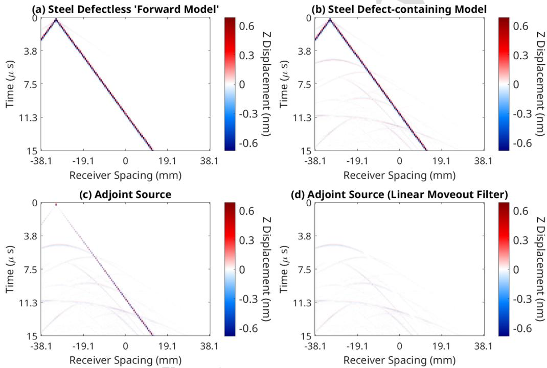
Figure 4: Space-time Signals for Source 12 in Numerical 5 MHz phased-array from (a) Defect-free and (b) Defect-containing Models. (c) The adjoint source evaluated from (a) and (b). (d) The filtered adjoint source.
