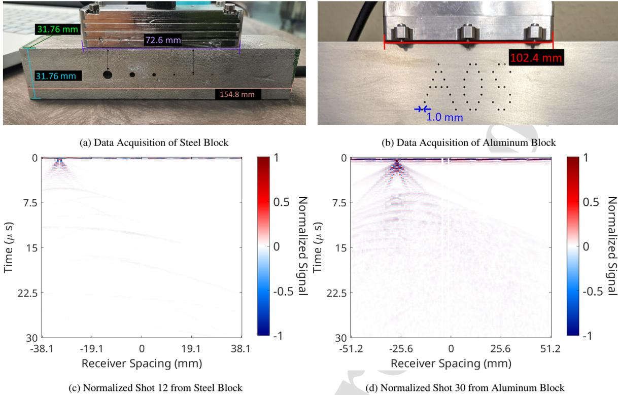
Figure 2: Data acquisition for steel (a) and aluminum (b) blocks. Shots in the FMC for steel (c) and aluminum (d) datasets.
