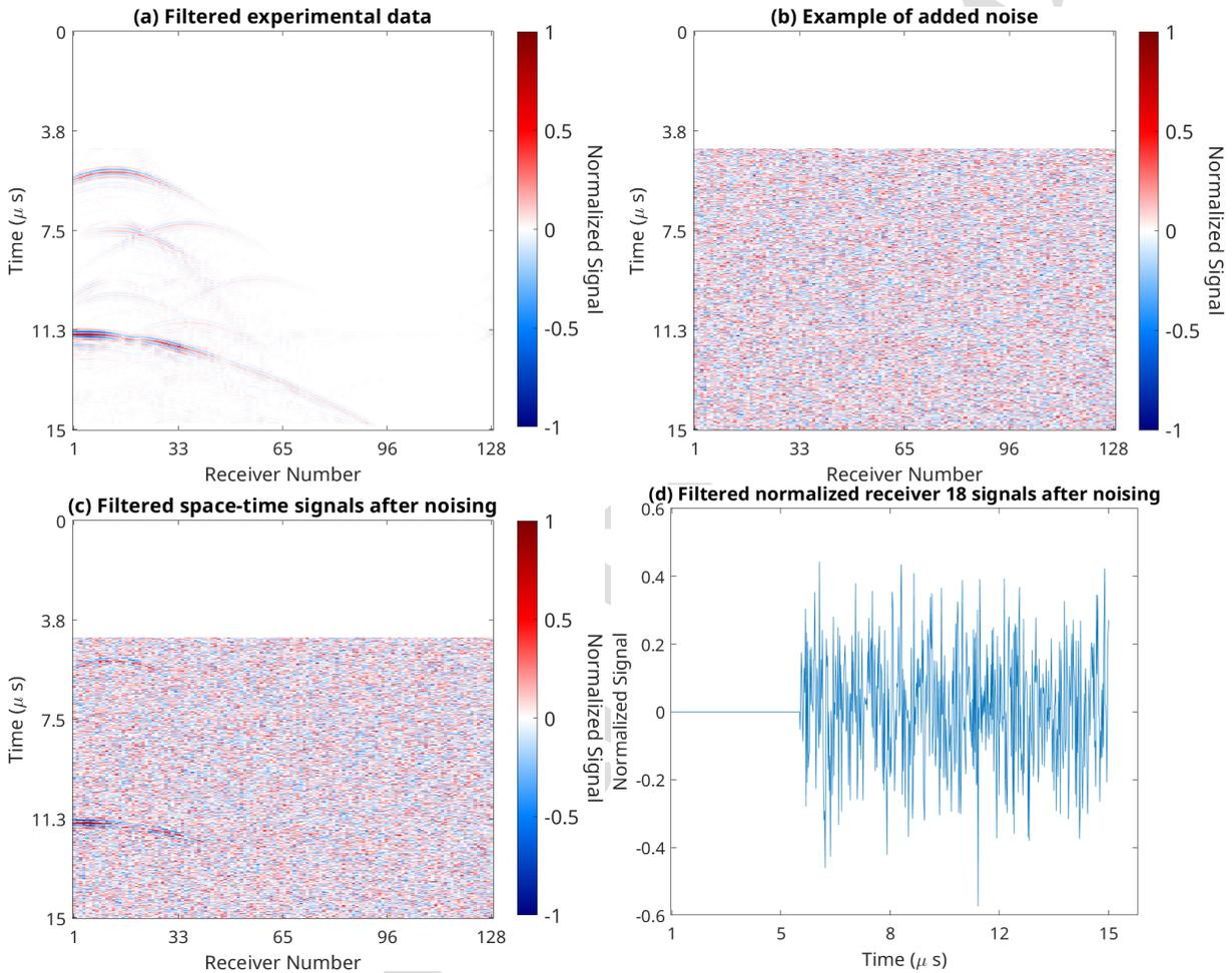
Figure 7: Noise addition process for “noisy” steel dataset: (a) filtered normalized ultrasound data from source 1, (b) example noise added to each source, (c) example “noisy” space-time signals for source 1, and d) example “noisy” 1-D signal for source 1 receiver 18 combination.
