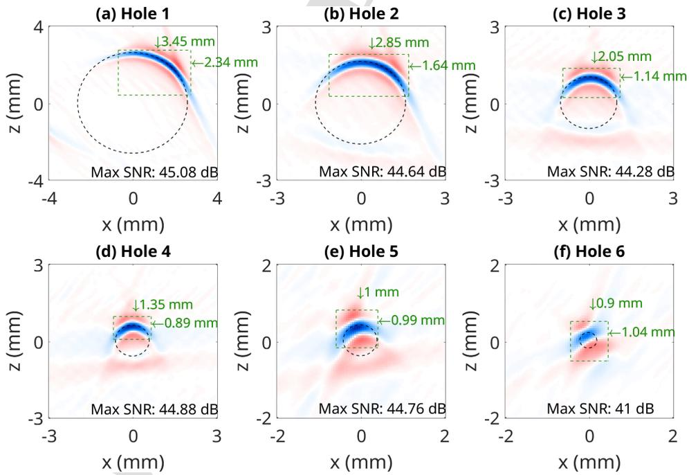
Figure 14: Zoomed in numerical steel images for each hole within  $I_{TFM}$ .
