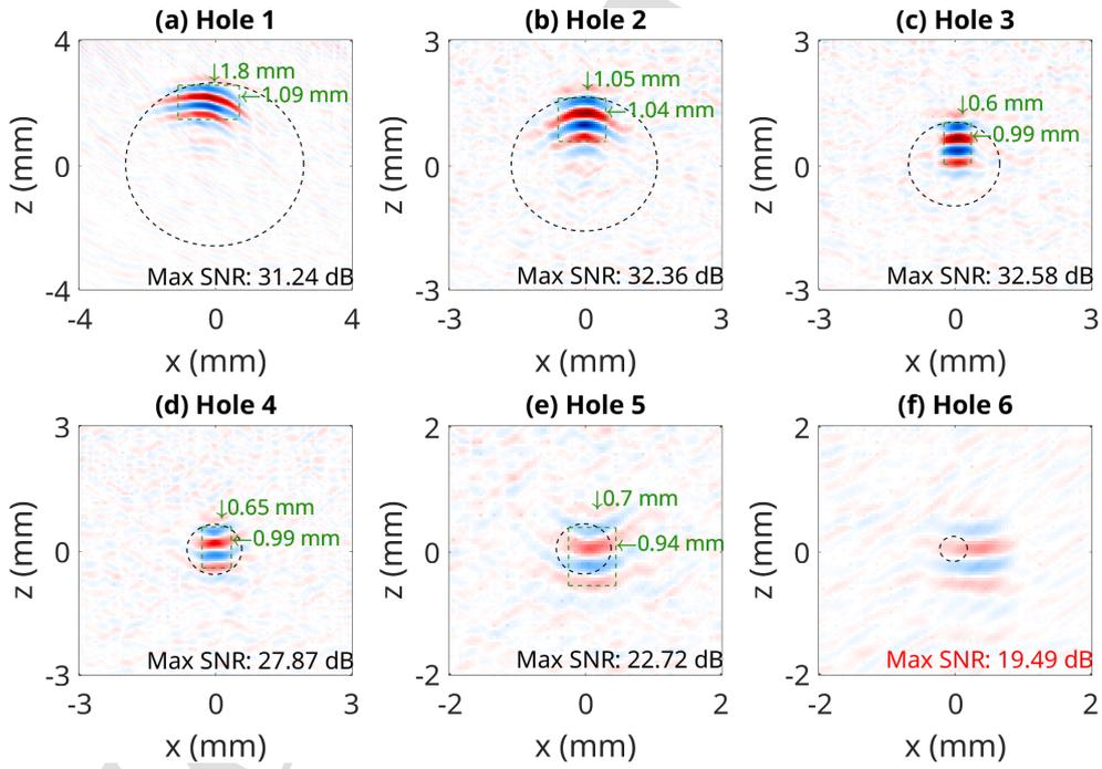
Figure 25: Zoomed in Experimental Steel Images for each hole within:  $K'_p$
