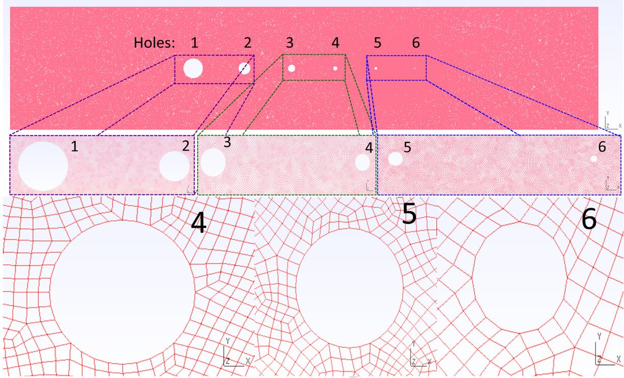
Figure 3: Externally generated mesh in Gmsh application
