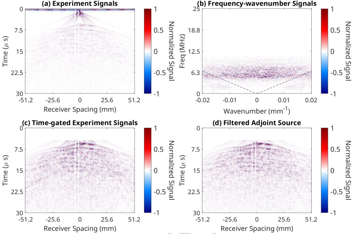
Figure 8: Example filtering of 5 MHz ultrasound data for source 64. (a) Unfiltered time-space and (b) frequency-wavenumber signals and filtering zone. (c) The time-domain signals with time gating. (d) The fully filtered adjoint source.
