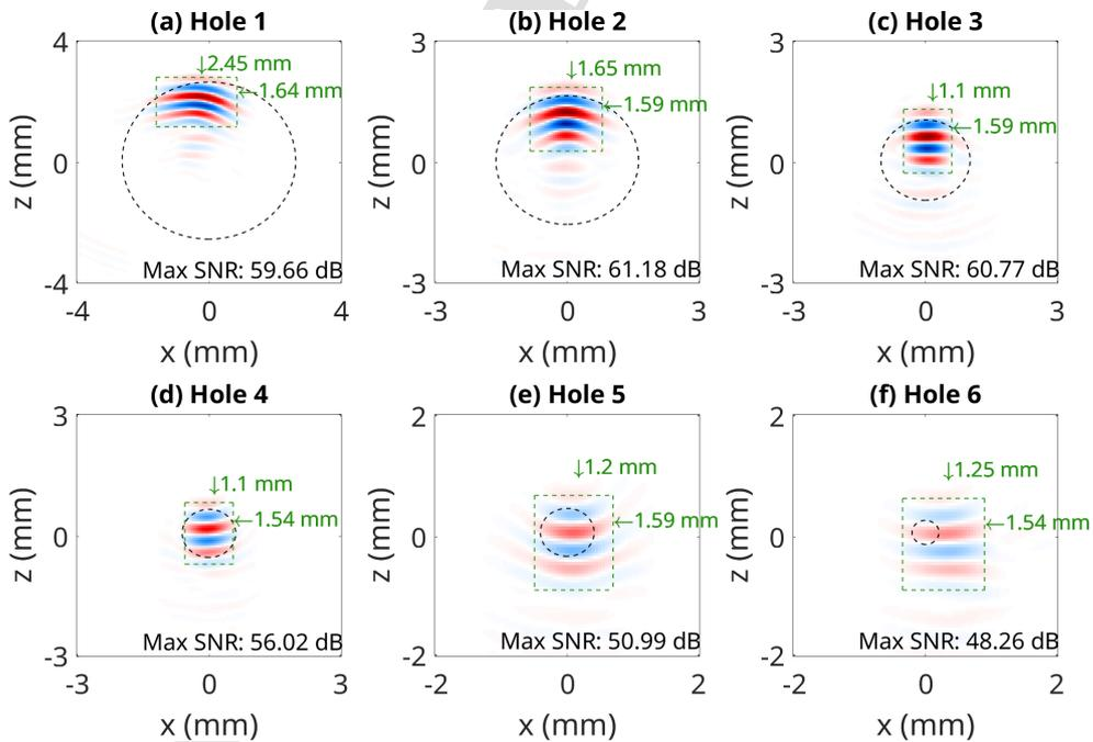
Figure 16: Zoomed in experimental steel images for each hole within  $K_{V_p}$ .
